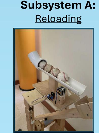
The stepper motor turns a three-prong rotor 120 degrees allowing for one ball to be released at a time.
