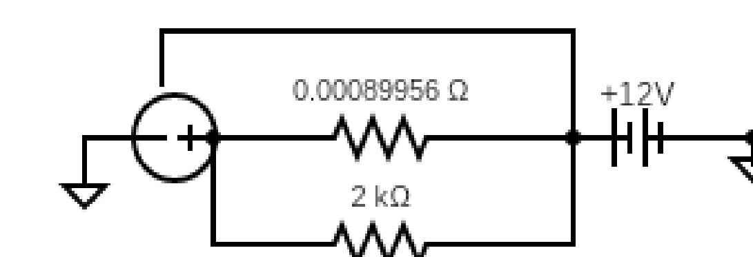
Figure 2: Circuit Diagram for parallel circuit to measure output. DC source represents alternator, wire going into the top represents the excitation charge
