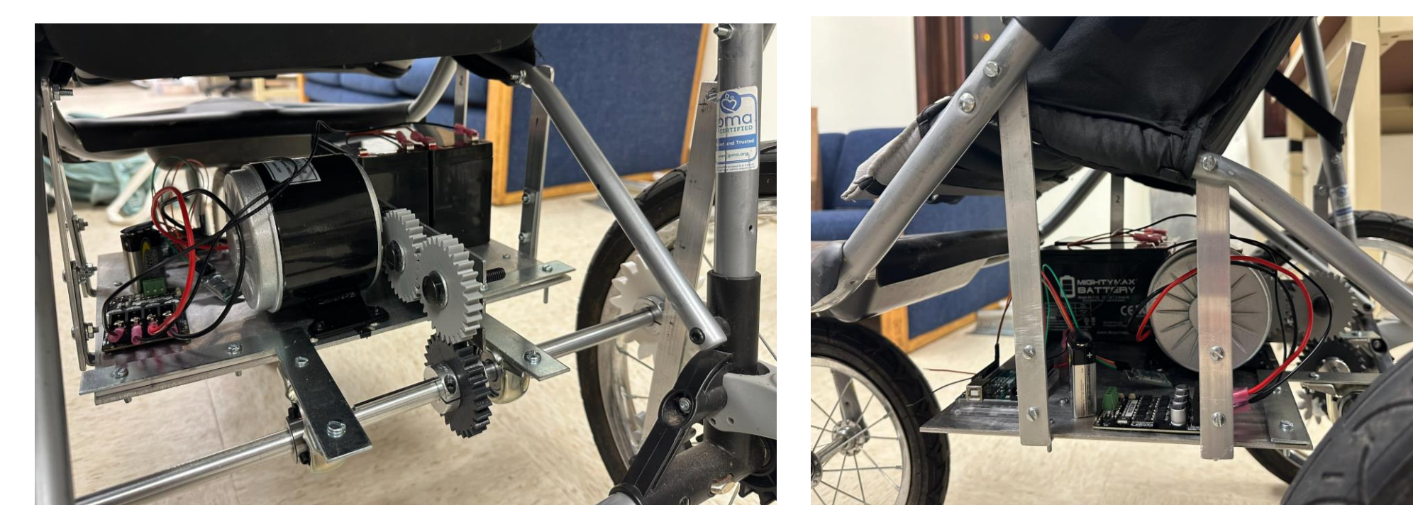
The final design highlighting the mechanical system and the electrical power system mounted in the undercarriage. Also pictured is a lever and gear that allows the user to disengage the power drive system.
