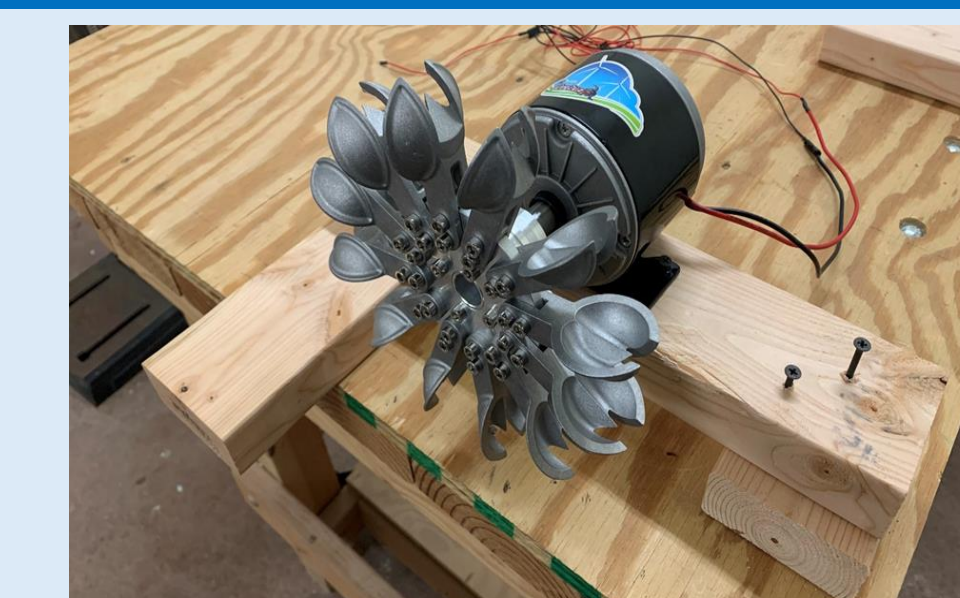
Figure 7, First design for turbine stand.
